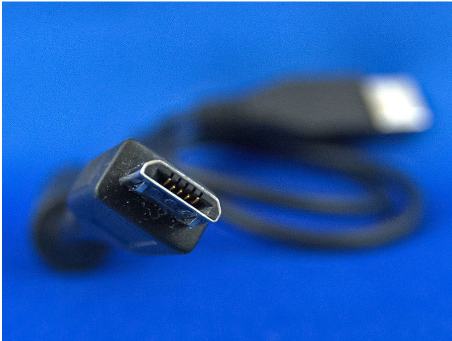
Figure 2-7. Micro USB B plug
