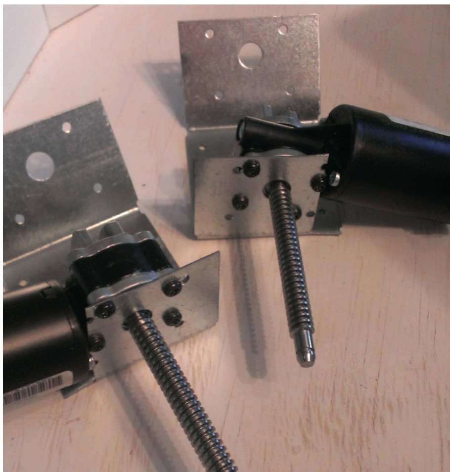
Figure 7-8. Motors attached to mounting brackets
