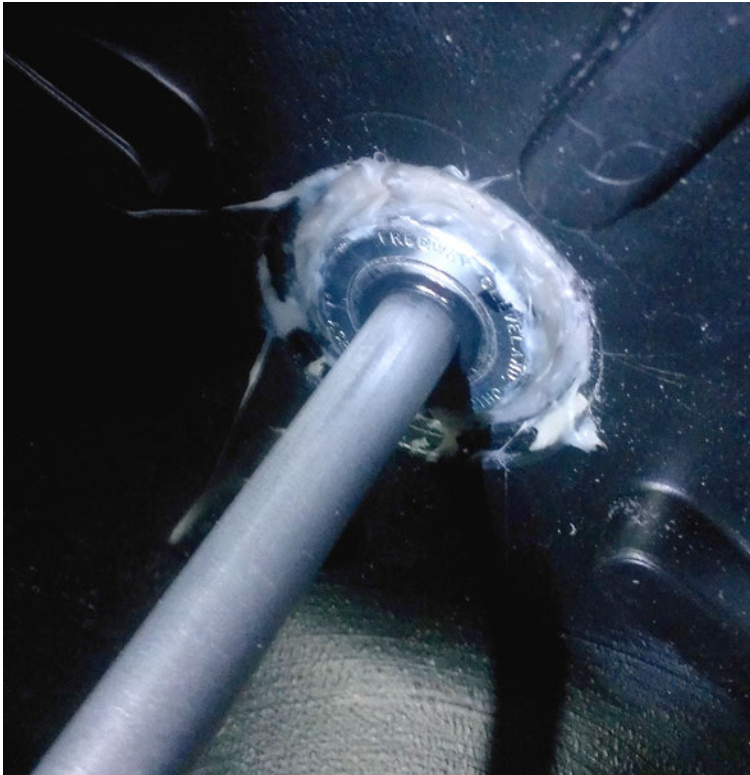
Figure 7-15. Bearing and axle attachment
