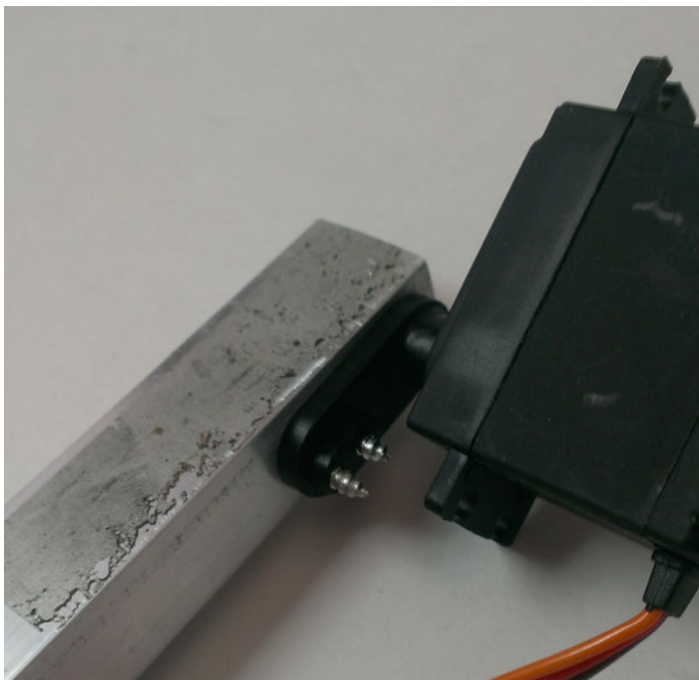
Figure 7-19. Arm attached to servo horn
