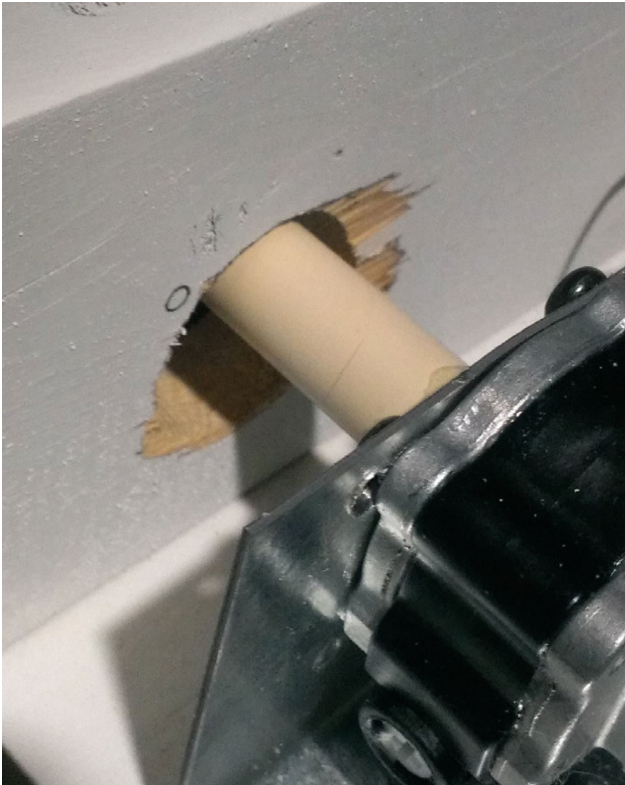
Figure 7-5. Hole for rear axle
