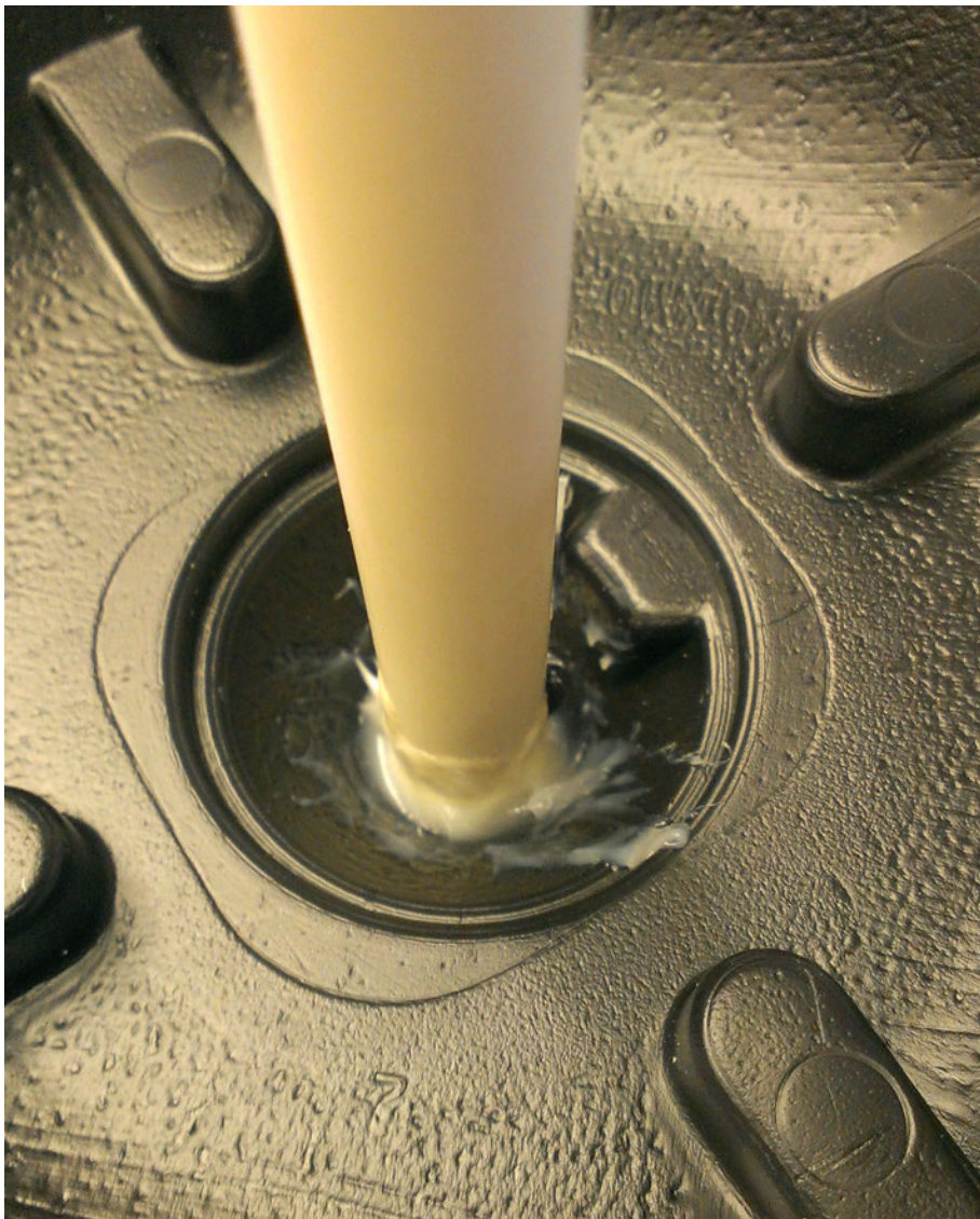
Figure 7-12. Axle pipe attached to wheel
